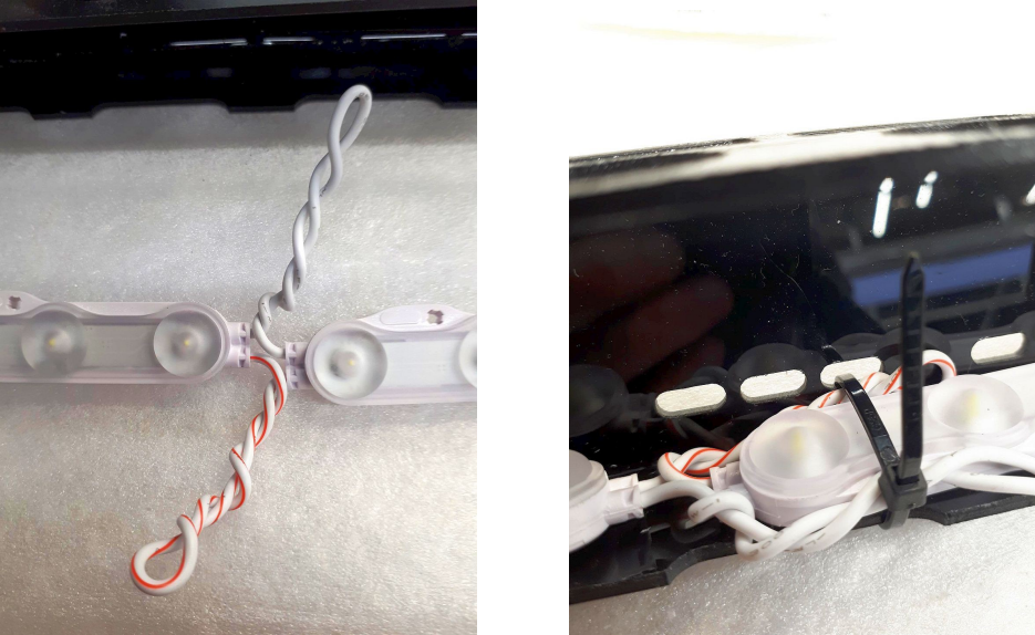
HOW TO BUNDLE EXTRA WIRING BETWEEN MODULES TO THE LOOPS AND STRING WITH ZIP TIES
